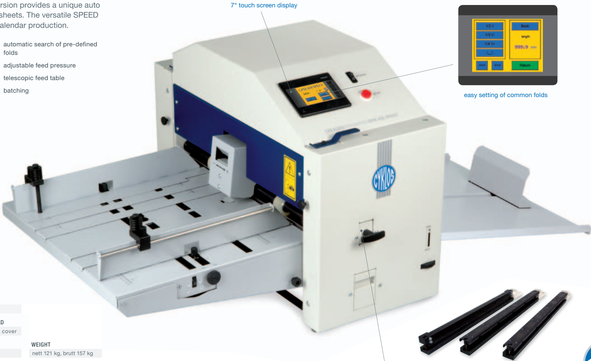
easily exchangeable creasing, perforating and punching tools
